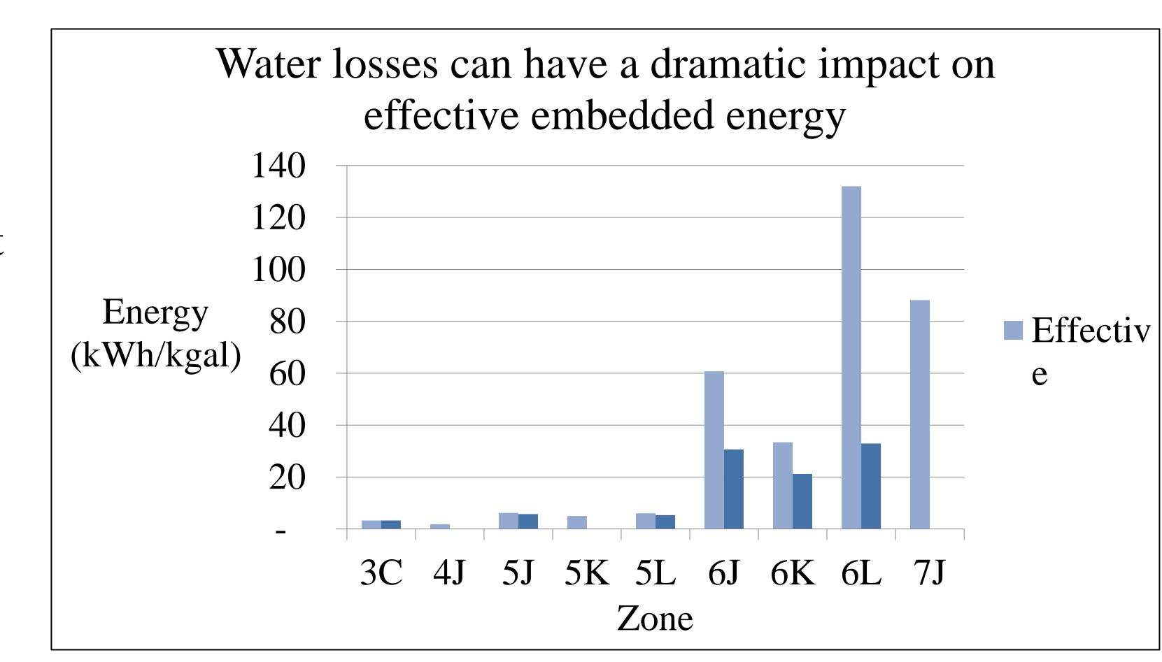
Figure 4: Comparison of Effective Embedded Energy (based on water customers receive) and Actual Embedded Energy (based on water pumped). The difference is the energy penalty due to water losses in the distribution system. It should be noted that zones 4J, 5K and 7J do not depict Actual Embedded Energy bars because of inaccurate data.
