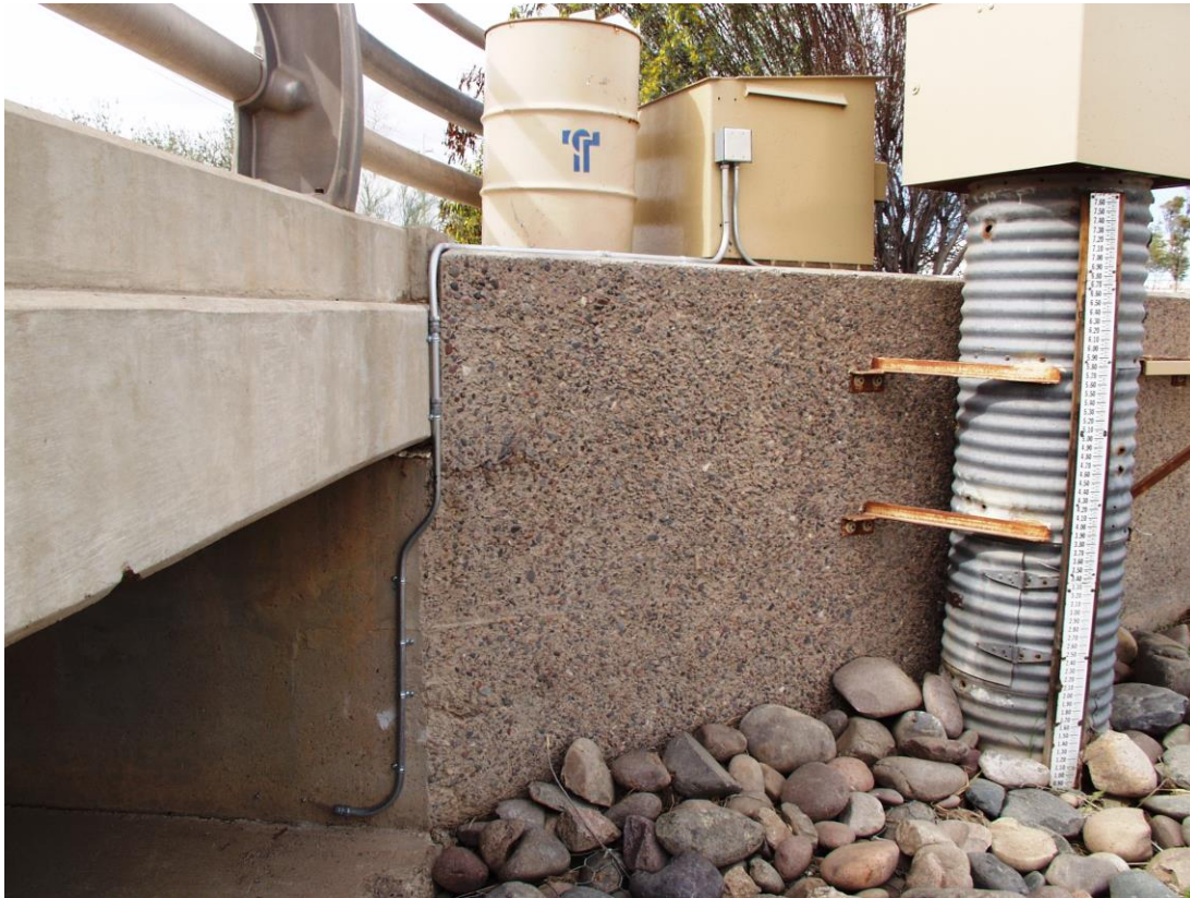
Stream flow gauge along Indian Bend Wash
