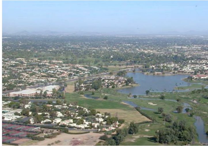
Figure 2.9. Riparianization in Scottsdale, AZ. In the foreground is the Indian Bend Wash floodway, but expansive areas of green vegetation can be seen far beyond the channel owing to redistribution of water onto residential and commercial landscapes.
