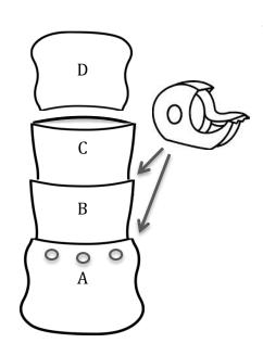
$4^{\rm Seal\,parts\,A,\,B,}$  and C with tape
