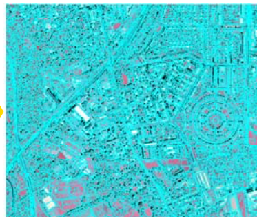
Figure 3. Pre-classified segmented image Polygons are raw objects used in succeeding classification procedure.
