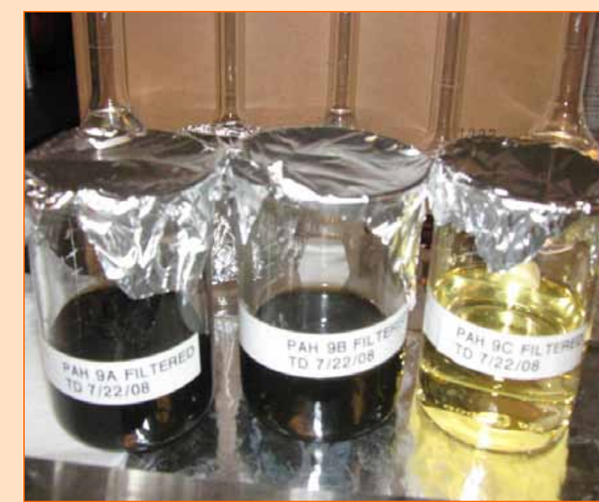
Fig. 3. Samples after ultrasonic solvent extraction.
