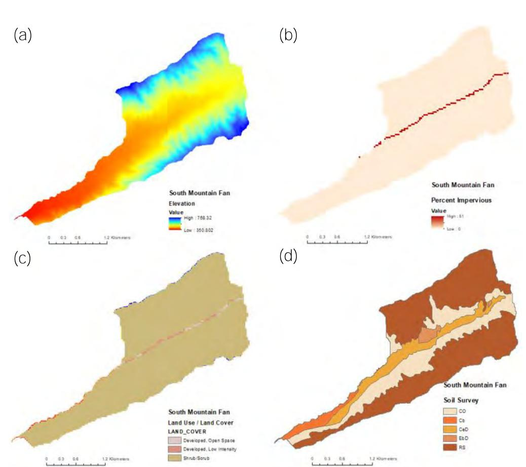
Fig. 5(a-d). South Mountain Fan (a) Elevation, (b) Percent Impervious, (c) Land Use/Land Cover, and (d) Soil Survey.
