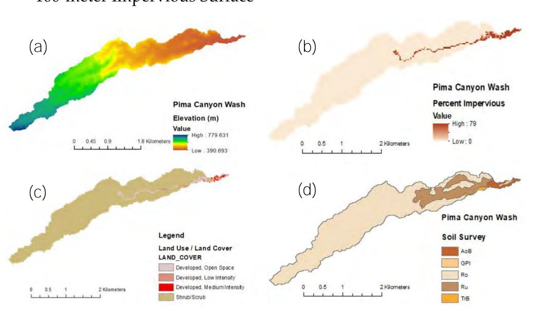
Fig. 4(a-d). Pima Canyon Wash (a) Elevation, (b) Percent Impervious, (c) Land Use/Land Cover, and (d) Soil Survey.
