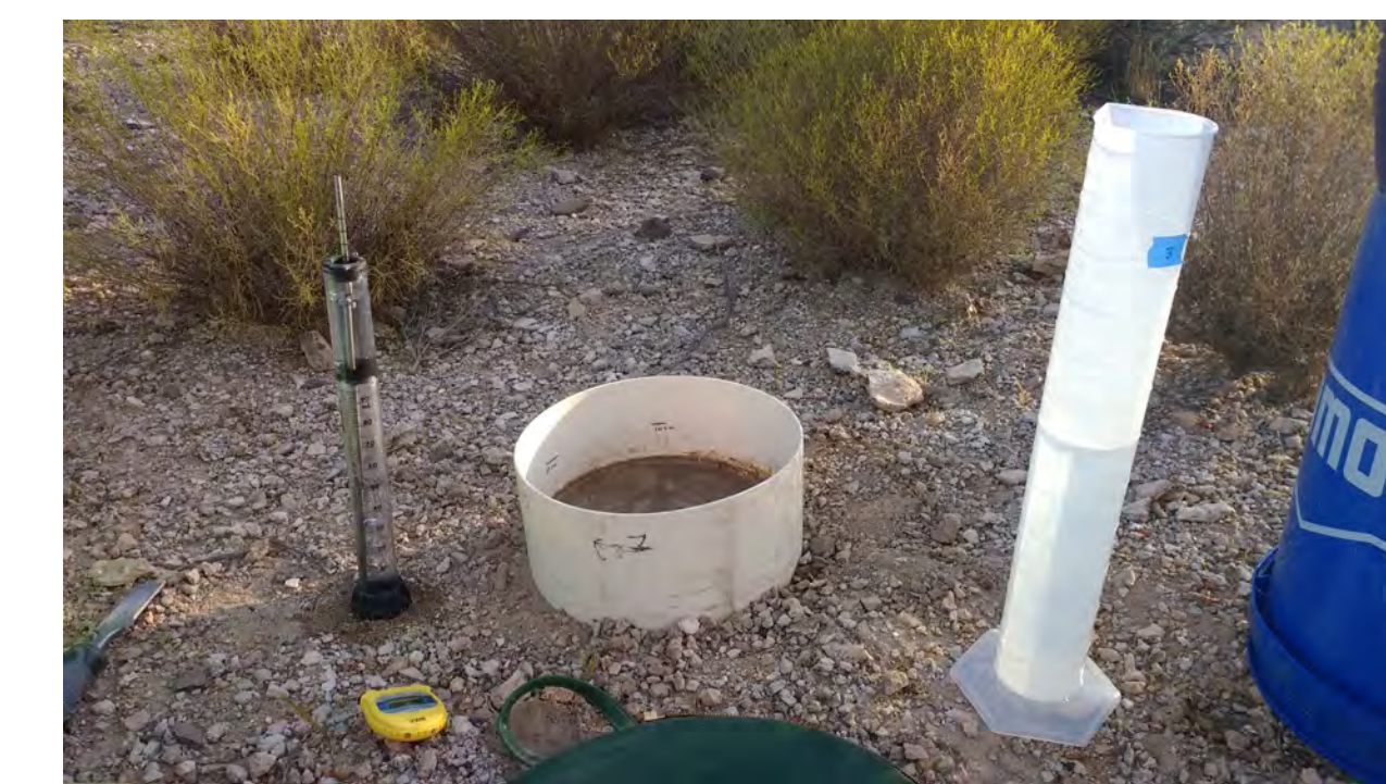
Tension infiltrometer for near-saturated infiltration rate
