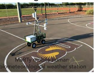
gure 4a (Left): We conducted hourly microclimate transects using the mobile human-biometeorological weather station "MaRTy" (left) to measure air temperature, relative humidity, horizontal wind speed and direction, six-directional radiation flux densities, and GPS location. Transects were conducted during daylight hours on hot, clear, calm summer days. MRT observations were analyzed across all sites, transects, measurement days, and observation times to determine shade coverage efficacy.
