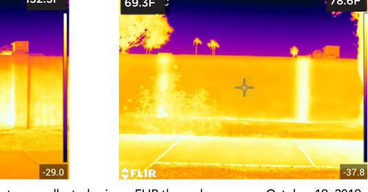
Figure 3c: Wall 24, surface temperatures, collected using a FLIR thermal camera on October 19, 2019 (Sky Harbor high air temperature 86F, low 60F, Sunrise: 6:35am Sunset: 5:50pm.) Structural concrete columns and ground beams showed highest night time temperatures
