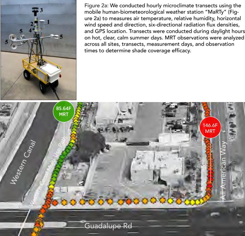
Figure 2b: Mean radiant temperatures collected using MaRTy (see figure 2a) at Western Canal Path at 8am on September 12, 2019 with high at Sky Harbor of 102F and low 80F, sunrise 6:09am and sunset 5:38pm.
