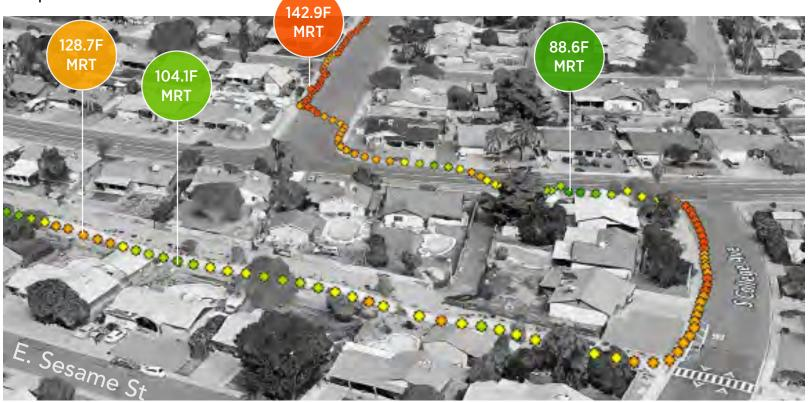
n radiant temperatures collected using MaRTy (see figure 2a) at El Paso Path at 8am o September 12, 2019 with high at Sky Harbor of 102F and low 80F, sunrise 6:09am and sunset 6:38pm
