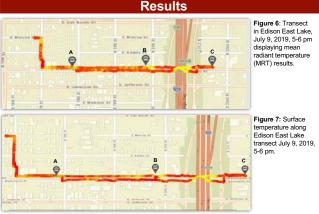
ArcGIS maps created from the data collected at the Edison East Lake transect. The maps were designed with a heat gradient along the transect to represent the fluctuations in mean radiant temperature (Figure 6) or surface temperature (Figure 7) along the route. There is more variability in the gradient in the MRT than surface temperature as more variables are integrated for MRT (includes both solar and infrared radiation).
