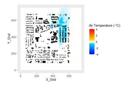
City of Phoenix is in the process of redeveloping the Edison Eastlake community, with one goal being to improve thermal environments for its residents. This project uses microscale atmospheric modeling to quantify the thermal conditions in the neighborhood before redevelopment, validate the model based on observations within the neighborhood, and then use the validated model to explore the thermal environment implications of various redevelopment designs. The value
