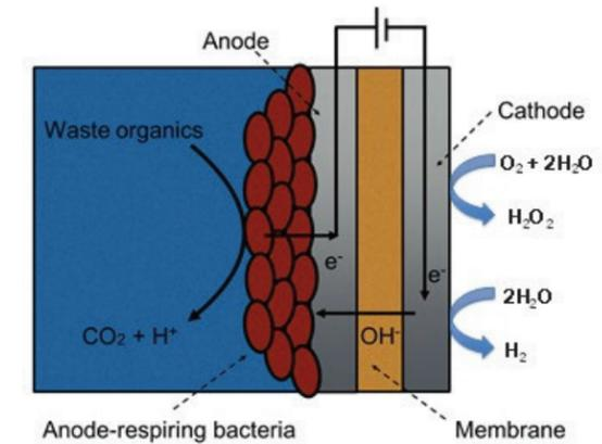
Figure 2: Schematic of an MxC to produce H<sub>2</sub> or H<sub>2</sub>O<sub>2</sub> from organics in dairy wastewater.
