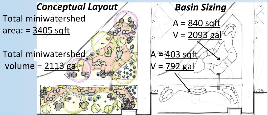
Using one 'mini watershed', volume calculations were used to determine the size of GI/LID techniques. This site allowed for direct reuse water harvesting basins to capture all available rainfall. However, other areas within the Campus are limited in area and require additional techniques (in form of a treatment train) to fully capture available runoff.
